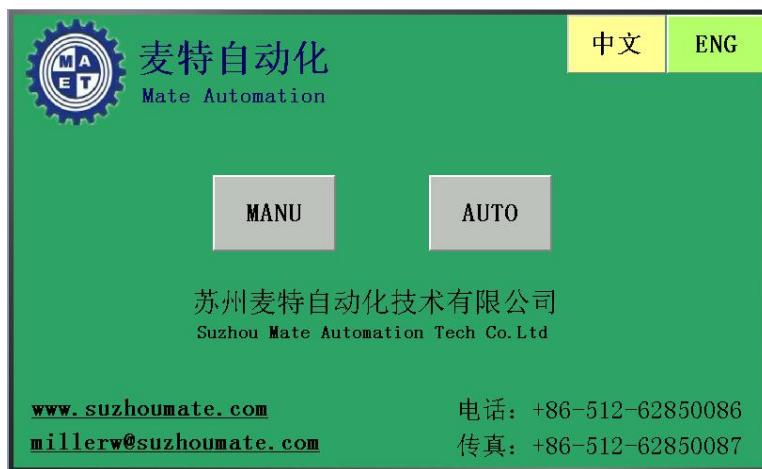
Press “MANU” button, it will shows following page, this page is used for only manual control the machine movements.
